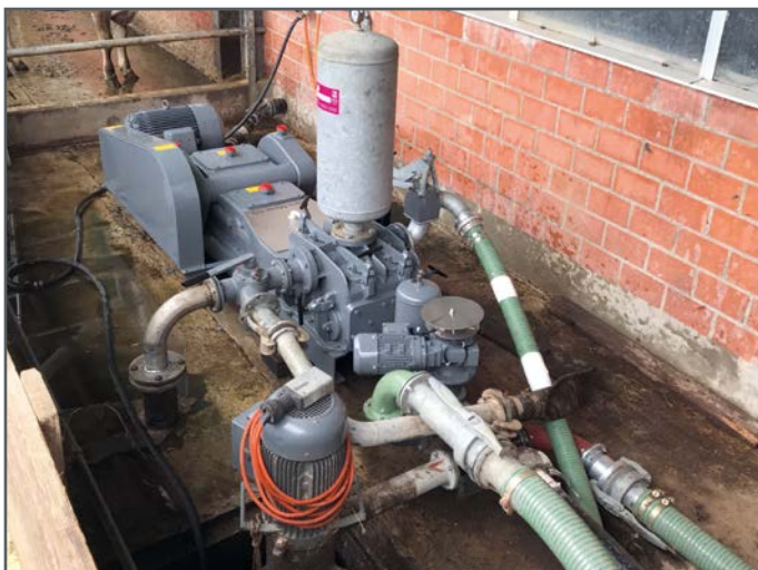
H-303-OSG2, E-Motor, Saugrohrmixer
